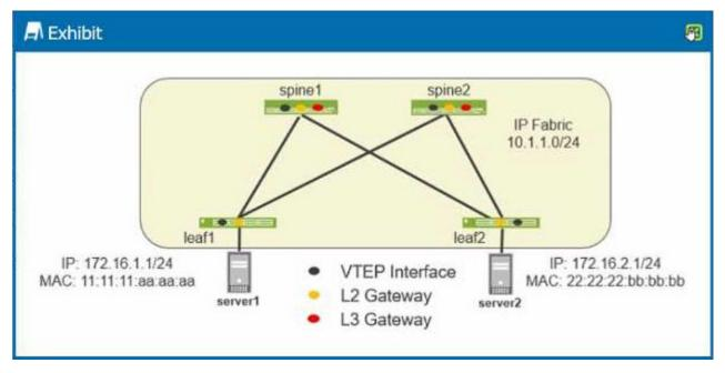
You have implemented an EVPN-VXLAN data center. Device served must be able to communicate with device server2.
