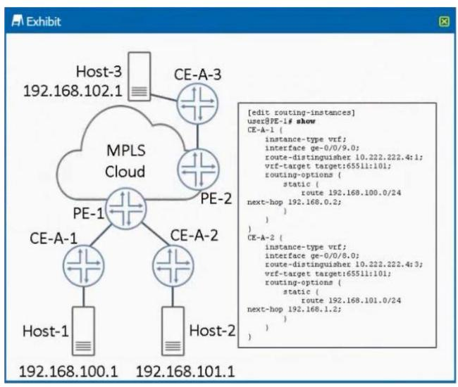
Referring to the exhibit, there is an Layer 3 VPN setup that connects sites CE-A-1. CE-A-2 and CE-A-3 together Host-1 can communicate with Host-3. but Host-1 cannot communicate with Host-2 What must you do to solve the problem?
