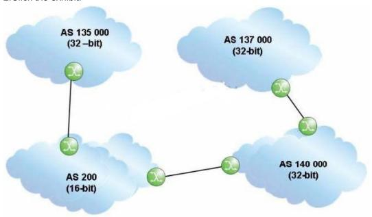
An update travels from AS 135000 to AS 137000, traversing both 32-bit and 16-bit AS paths. What will the AS Path be when the update reaches AS 137000?
